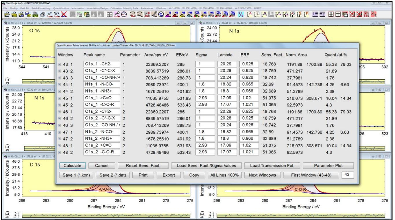
**Fig. 1** Screen shot of the quantification table: with the button 'All lines 100%' or 'Par. Lines 100%' the calculation of the at-% values (column: Quant./at.%) takes all lines or the lines with the same batch parameter, the figure illustrates the 100% normalization of the windows 43, 44 and 45 (parameter = 1) and 46, 47 and 48 (parameter = 2)
