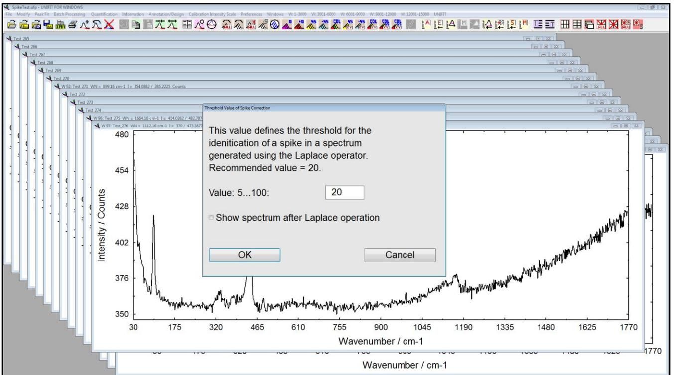
**Fig. 4.** Screen shot: Setting for the threshold for the identification of the spikes, option: show the spectra after Laplace operation
