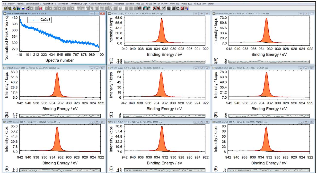
**Fig. 2.** Validation experiments of the stability of the mono source: measurement time: 6 hours, number of spectra: 1100, every 128th spectrum standard window is displayed, a strong reduction of the intensities can be observed (parameter plot: top, left)
