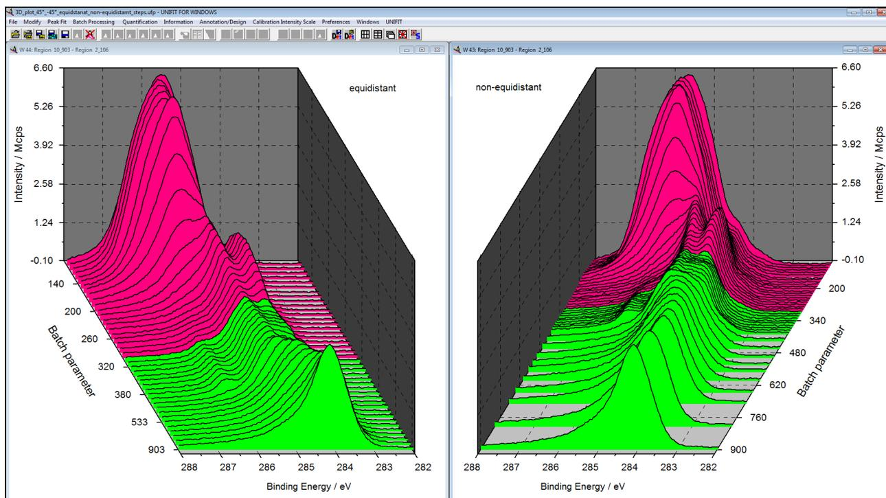
**Fig. 4.** Left: Plot 3D Waterfall -45° with equidistant parameter steps, right: Plot 3D Waterfall 45° with non equidistant parameter steps (true parameter step width)
