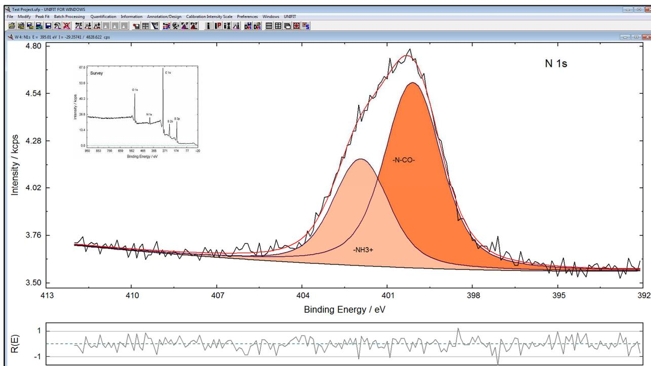
**Fig. 6.** Screen shot of a standard window of UNIFIT 2012 (fitted N 1s spectra), embedded the corresponding survey
