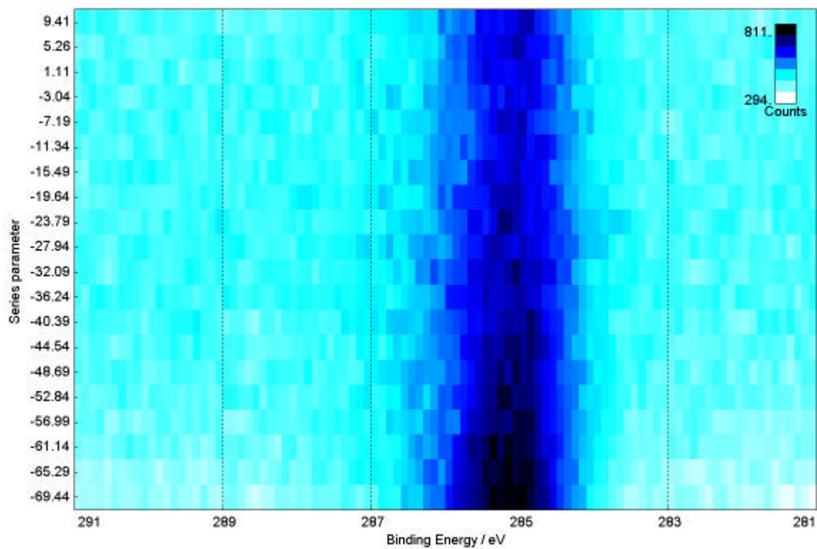
Fig. 4. A 3D Colour plot of the C 1s contamination peak using UNIFIT 2005
