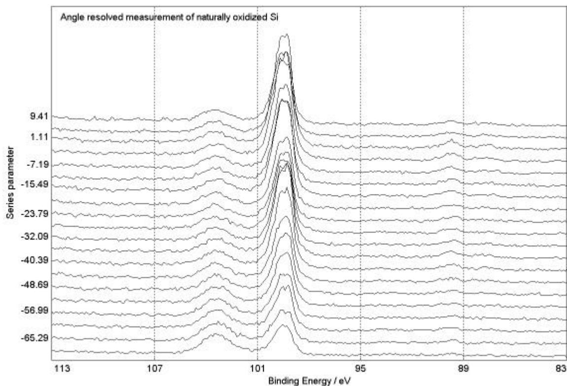
Fig.. 1. 3D Waterfall 0° plot of an angle resolved measurement of a naturally oxidized Si wafer using UNIFIT 2005. The exported bitmap graphic was inserted in this Word document
