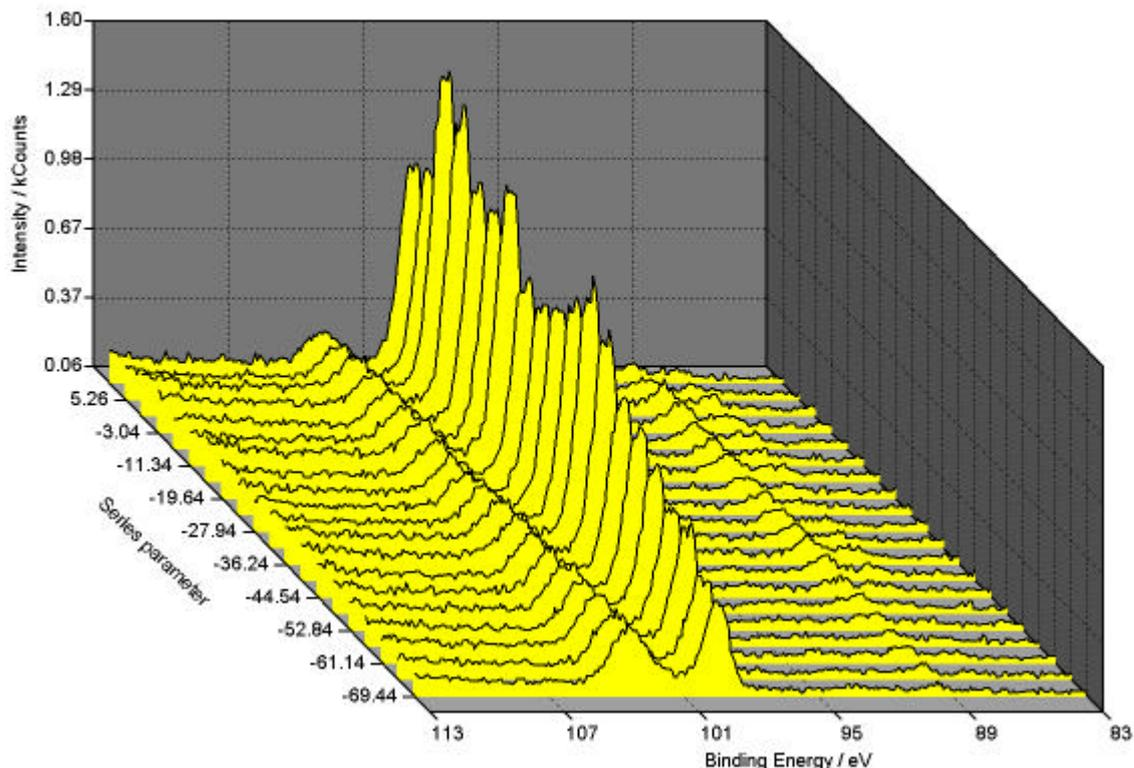
Fig. 3. 3D Waterfall -45° plot of an ARXPS measurement of naturally oxidized Si using UNIFIT 2005
