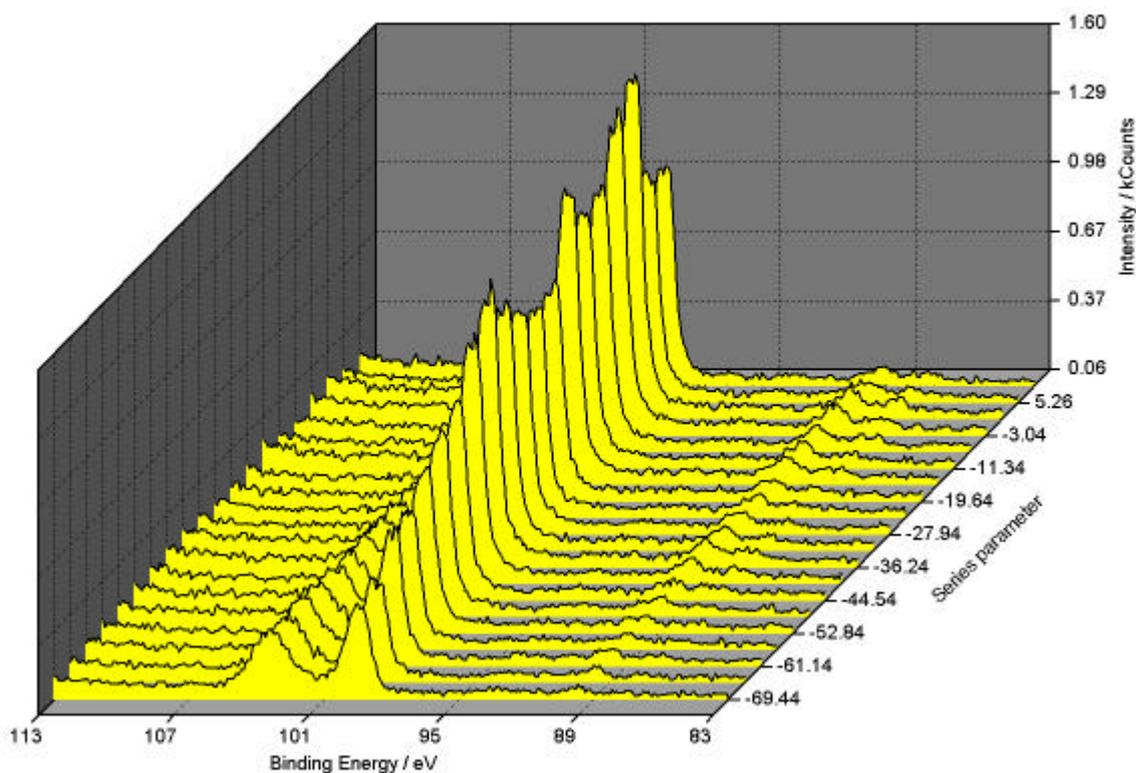
Fig. 2. 3D Wasserfall 45° plot of an ARXPS measurement of naturally oxidized Si created using UNIFIT 2005
